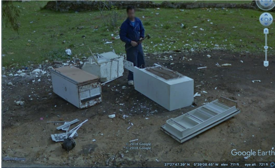
Google Street View of scavenger "station" and man harvesting metal and parts from old refrigerators. Note compressor in foreground and oily soil from long periods of this type of activity. This is where tracker enable CRT ES137294 ended its journey in the town of Carmona, in Andalucía. It could also be a location of illegal releases of CFC gases. Map data: Google, DigitalGlobe.
