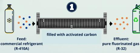
This prototype is highly efficient for the separation of R-410A, with high performance in the selective recovery of high purity R-32. With simple adjustments, it could be applied to other F-gases. It has low energy and maintenance requirements, and it is easy to apply in a waste management facility due to the small amount of space required, and due to its modularity and scalability.
